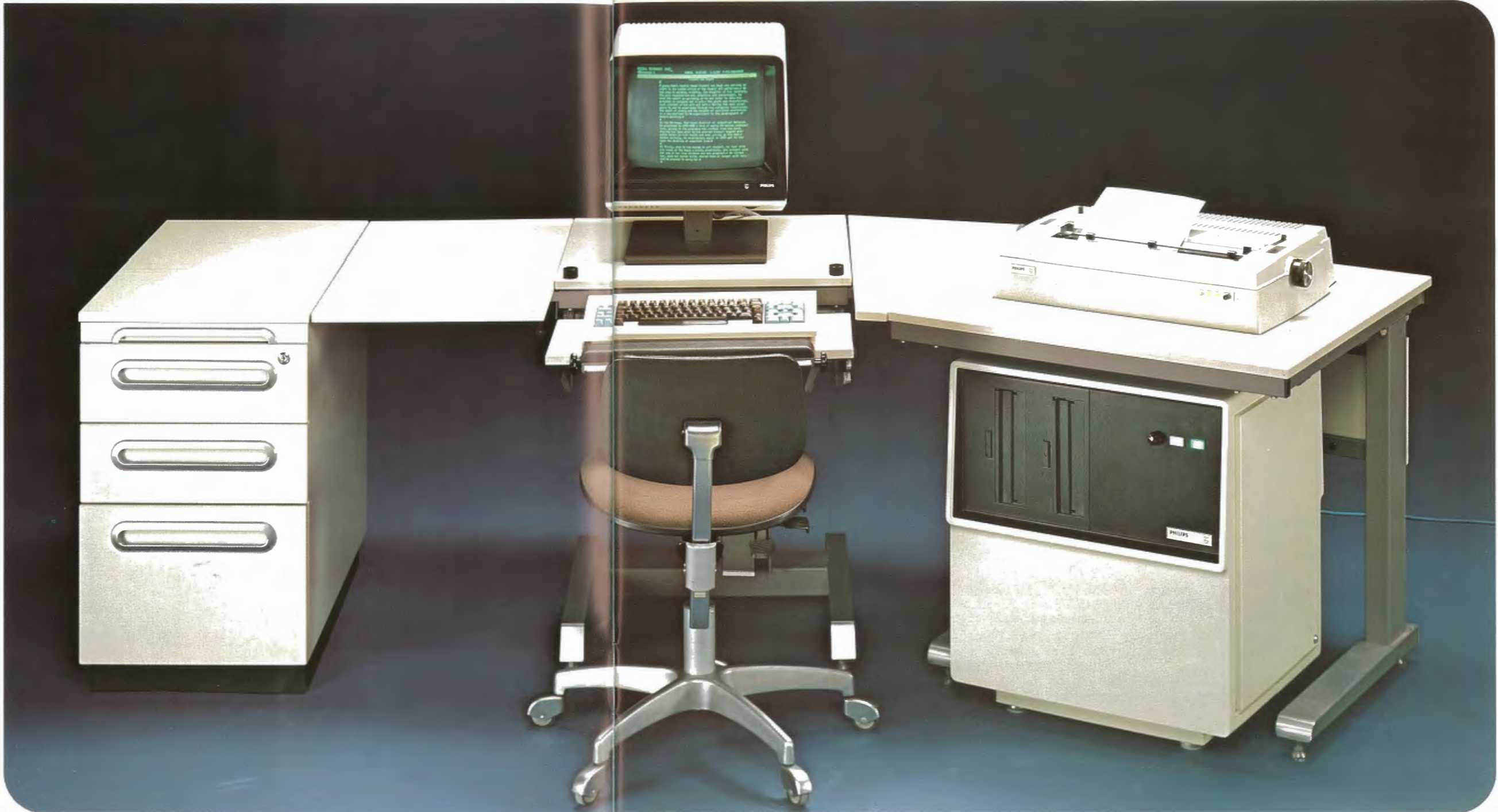
By means of dual disk drive units, information can virtually instantaneously be recorded on to or recalled from the flexible disks. Information can be sent and received via the telephone (background function) while the operator carries out other tasks (foreground function).
