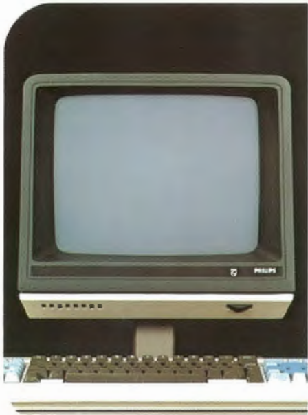
A standard typewriter keyboard is used for typing text on to the screen of the VDU (Video Display Unit). The keyboard and VDU are separate, and independently adjustable, for maximum operator convenience.
